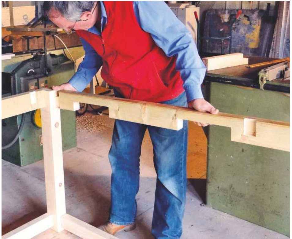
▲ Pic.3 The table is of standard construction except for the housing of the vices. The stopped housings hold cross-members, while the cut-outs accommodate the vices
